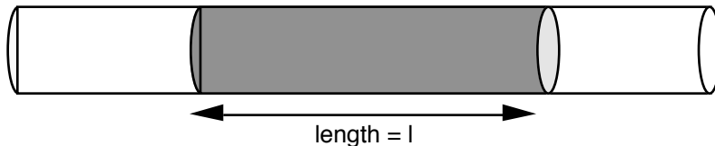
After time \Delta t , electrons have filled a volume V (shaded region.)
